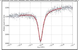
FIGURE 4: Three photon CPT dark resonance with 794 nm and 866 nm lasers locked on the OFC referenced to the clock laser. The contrast of the line is 21% and its linewidth is  $51~\rm kHz$ .
