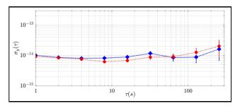
FIGURE 2: Allan deviation of the 12 MHz beatnote between comb mode N+4 and  $\nu_1$  (red  $\bullet$ ) and the reference beatnote at 260 MHz (blue  $\Phi$ )
