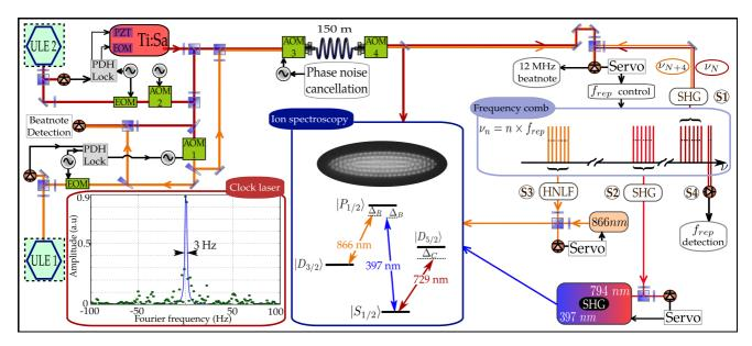
FIGURE 1: Locking scheme and experimental set-up of the locked 729 nm-laser and stability transfer to other sources via OFC. Inset: Beatnote between the two laser arms exhibiting a Gaussian linewidth (FWHM) of 3 Hz with a resolution bandwidth of 1.5 Hz. The central part of the Figure illustrates the ion crystal and energy level scheme of Ca<sup>+</sup>-ions.
