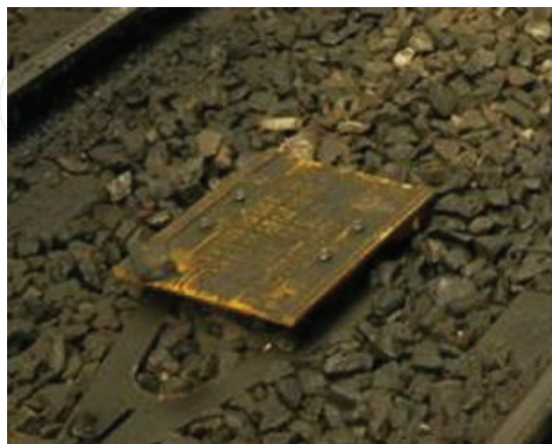
Figure 3. Example of balise mounted on the track.
