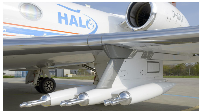
Figure 18 – PMS carrier, simulation model and hardware
