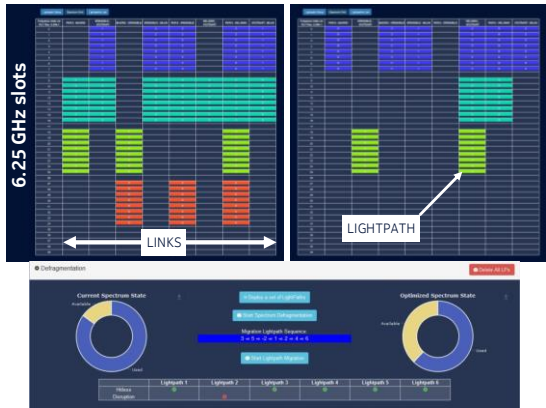
Fig. 5: Spectrum grid allocation before (above left) and after (right) execution of defragmentation VNF, GUI (below).
