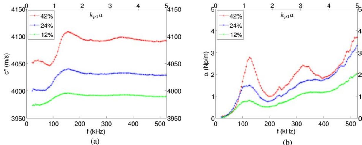
**Fig. 11.** Variations of velocity and of attenuation versus frequency and versus  $k_{p1}a$  in the case of an incident pressure wave propagating in a mortar containing 12%, 24% or 42% of scatterers of radius 6 mm in the case of full-wave numerical results.
