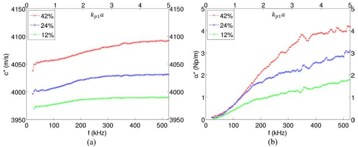
**Fig. 12.** Variations of velocity and of attenuation versus frequency and versus  $k_{p1}a$  in the case of an incident pressure wave propagating in a mortar containing 12%, 24% or 42% of scatterers of various radii in the case of full-wave numerical results.
