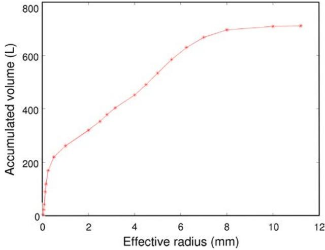
Fig. 1. Size distribution of aggregates for VeRCoRs concrete.
