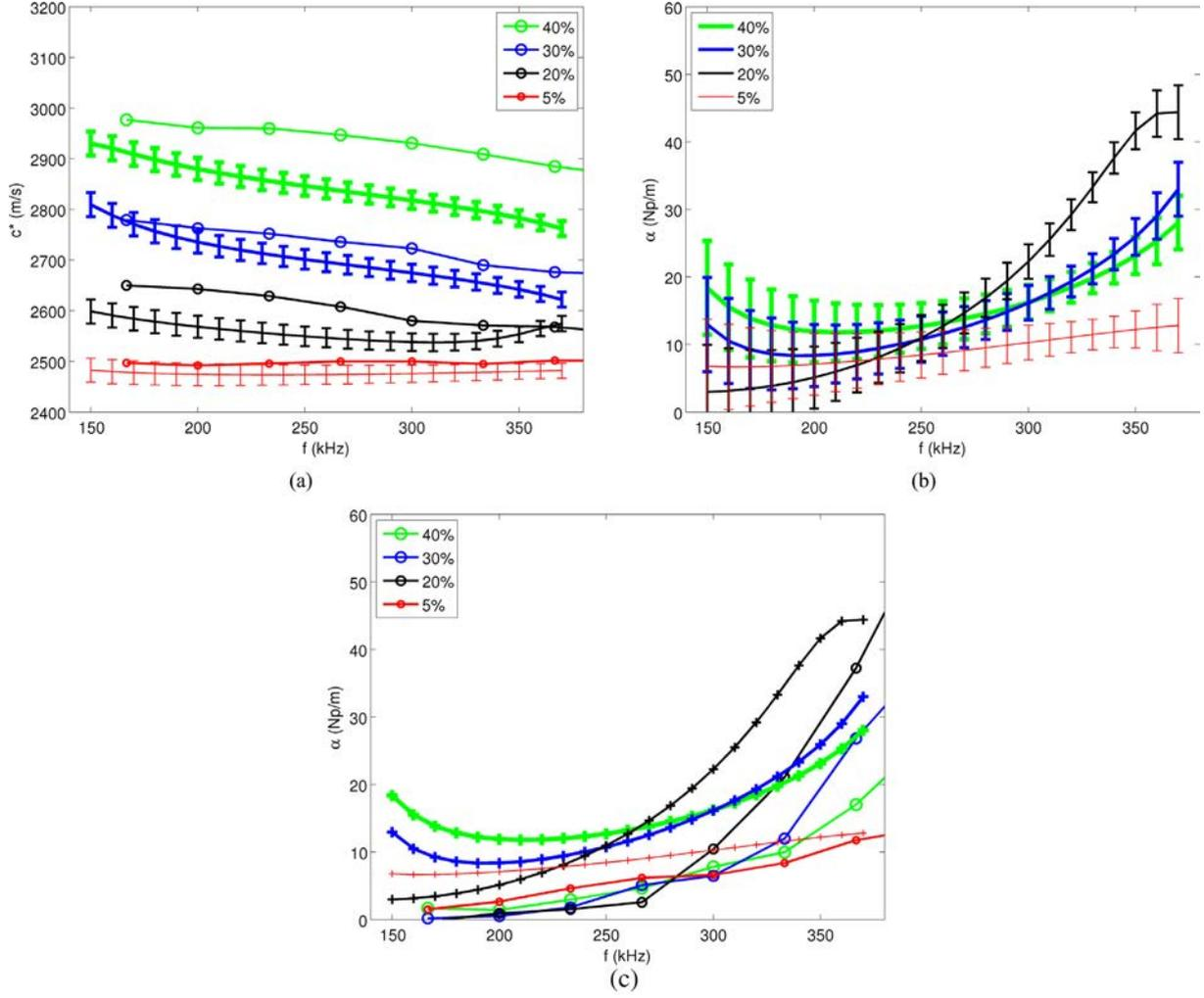
**Fig. 8.** Experimental (solid line with error bars or crosses) and numerical (solid line with circles) (a) velocity and (b)&(c) attenuation with respect to frequency in the case of pressure wave propagation in a medium composed of 5%, 20%, 30% and 40% of rods in resin. The measured attenuations in (c) are the same as the ones in (b), with the error bars removed for clarity.
