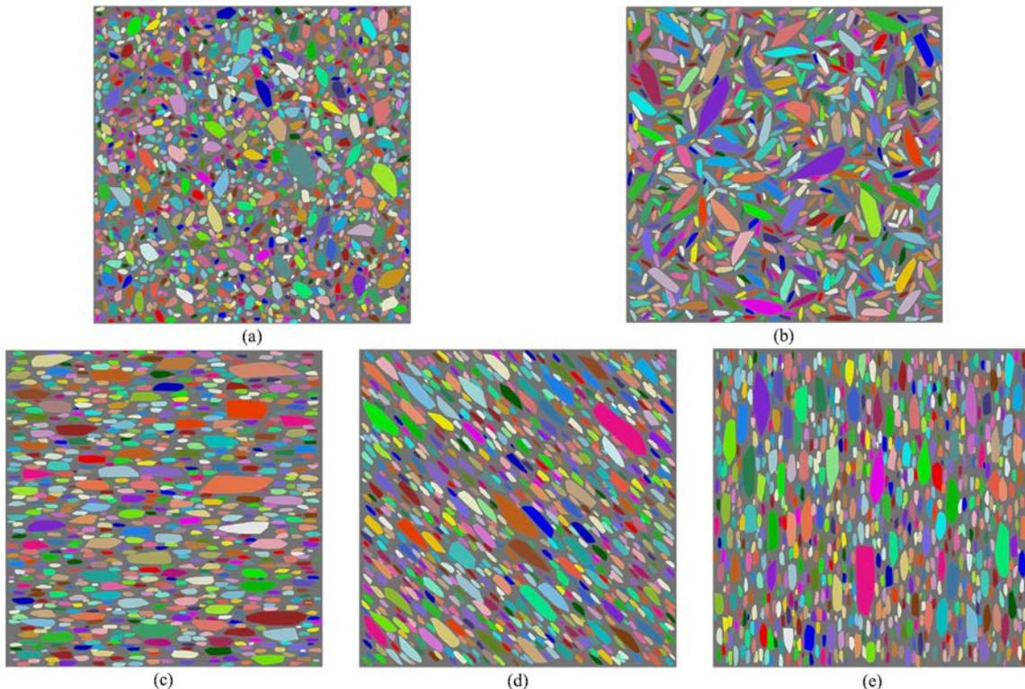
**Fig. 13.** Geometry of the mortar containing scatterers of polygonal shape. Polygons with a length over width ratio  $l/w$  of 3–4 with random directions (a), with a privileged direction of  $0^\circ$  (b),  $45^\circ$  (c) and  $90^\circ$  (d), and with a length over width ratio  $l/w$  of about 2 with random directions (e).
