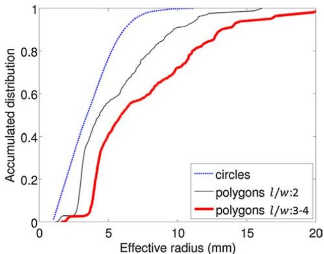
**Fig. 10.** Size distributions for the numerical cases with circles (dotted line) and polygons with a ratio  $l/w$  of about 2 (black solid line) and of about 3–4 (red solid line).  $l/w$  is defined by the ratio of the longest dimension of a polygon and the largest width in its perpendicular direction. (For interpretation of the references to colour in this figure legend, the reader is referred to the web version of this article.)
