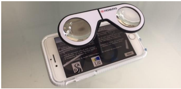
Figure 3 - A Homido mini VR viewer installed on a smartphone for stereoscopic view of the 3DAV Explore application
