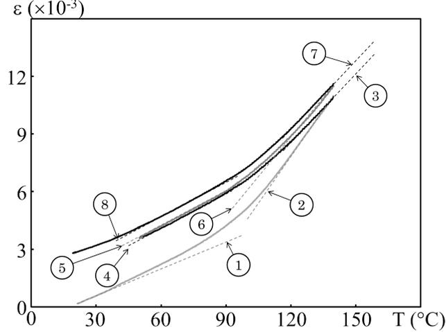
Figure 3: Thermal longitudinal strain  $\epsilon$  versus temperature  $T$  for cyclic thermal loading above room temperature. The dashed lines correspond to linear zones of the thermogram, referred to through numbers (see text). Grey lines: heating; Black lines: cooling.
