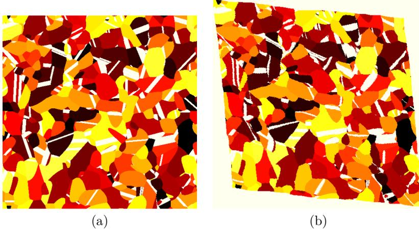
Figure 14: Johnson–Mehl model with “weakest-plane” transgranular cracks (JM-TW) under shear loading  $\bar{\varepsilon}_{xy} = \bar{\varepsilon}_{yx} = 10\%$ : 2D cut along the  $(x, y)$ -plane of the undeformed (a) and deformed microstructure (b). Cracks in white, grains in yellow, orange, red and black.
