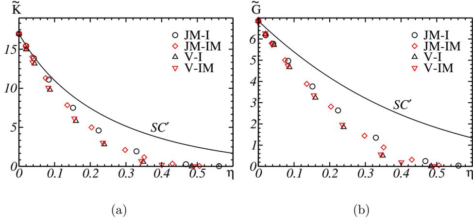
Figure 18: Bulk modulus  $\tilde{K}$  (a) and shear modulus  $\tilde{G}$  (b) of polycrystals with intergranular cracks as a function of the crack density  $\eta$ . Black symbols: the presence of a crack is not correlated to the adjacent grains orientations; Red: cracks occur in-between misoriented grains. Circles and diamonds: Johnson–Mehl tessellation; triangles: Voronoi tessellation. Solid line: self-consistent estimate  $SC'$  for cracked hexagonal polycrystals.
