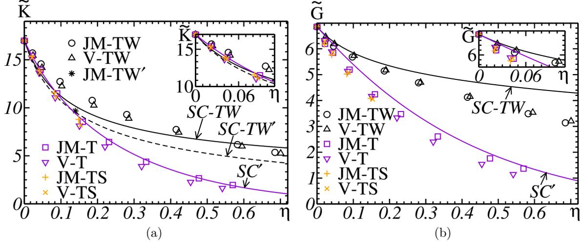
Figure 15: Elastic moduli of weak-plane (black symbols) and stiff-plane (orange symbols) transgranular crack models, as a function of the crack density parameter  $\eta$ , and compared to uncorrelated transgranular models (purple symbols). Solid lines: self-consistent estimates (SC-TW), (SC-TW') relevant to weak-plane cracked models and (SC'). Embedded graphs: enlargement around small crack density.
