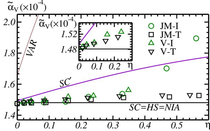
Figure 12: Continuation of Fig. 11: volumetric thermal expansion coefficient  $\tilde{\alpha}_V$ . Embedded graph: enlargement in the region  $\eta \leq 0.3$  for models (V-T) and (V-I), based on the Voronoi tessellation. Brown solid line: Gibiansky-Torquato upper-bound (VAR).
