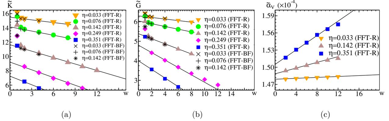
Figure 10: Influence of the crack width parameter  $w$  (in voxels unit length) on the effective elastic moduli (a-b) and thermal expansion coefficient (c) in a polycrystal (model JM-T) with transgranular cracks. Symbols: FFT data points using method FFT-BF (color symbols) and FFT-R (black signs), for various values of the crack density parameter  $\eta$ . Solid lines: linear fit in the range  $w \geq 2$ .
