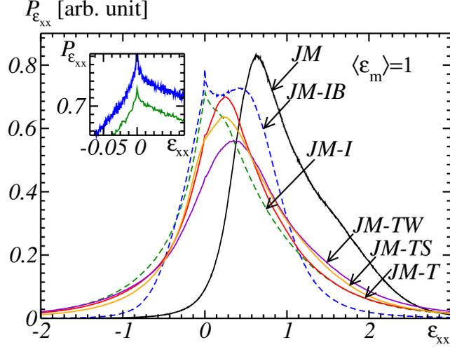
Figure 20: Histograms of the component  $\epsilon_{xx}$  in various cracked Johnson–Mehl models (colored curves) with  $\eta = 0.24$  and in an uncracked model (black solid line). Embedded graph: enlargement around  $\epsilon_{xx} \approx 0$  for models JM-IB and JM-I.
