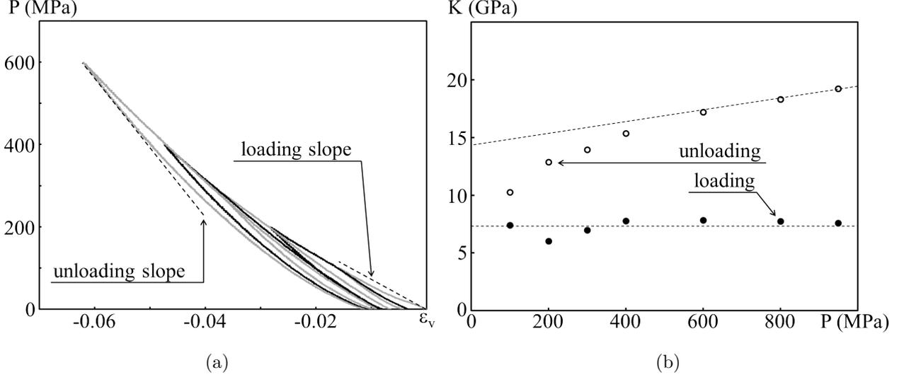
Figure 2: (a) Pressure  $P$  vs volumetric strain  $\epsilon_v$  recorded in hydrostatic cyclic compression. For legibility, the cycles at 800 and 950 MPa maximum pressure are omitted. (b) Loading and unloading slopes  $K$  versus pressure  $P$  defined in (a) vs the maximum pressure of the corresponding cycle.
