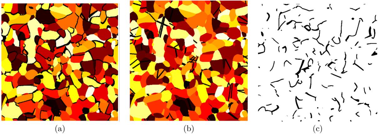
Figure 7: 2D sections of an anisotropic Johnson–Mehl tessellation with (a) intergranular and (b) transgranular cracks (black), denoted JMA-I and JMA-T respectively. Discretization:  $512^3$  voxels and  $w = 4$  voxels. The cracks take 10% (JMA-I) and 4% (JMA-T) of all voxels. (c) 2D section of a binary Johnson–Mehl tessellation, obtained by replacing the grains in (a) by an homogeneous matrix.
