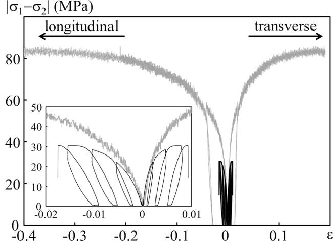
Figure 1: Principal stress difference  $|\sigma_1 - \sigma_2|$  versus logarithmic longitudinal or transverse strain  $\epsilon$  for uniaxial cyclic compression (in black) and triaxial compression (in grey). Negative strains are recorded by the longitudinal gauges, positive ones by the transverse gauges. The inset is a magnification of the  $[-0.02; 0.01]$  strain range.
