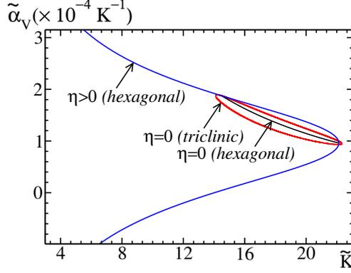
Figure 9: Effective thermal expansion coefficient  $\tilde{\alpha}_V$  as a function of the effective bulk modulus  $\tilde{K}$ . Solid lines: Gibiansky and Torquato’s upper and lower bounds (Gibiansky and Torquato, 1997) for the uncracked TATB polycrystal with triclinic anisotropy (red), Hashin formula (21) for hexagonal polycrystals (black), upper and lower bounds (26) for the cracked TATB polycrystal, with hexagonal approximation (blue).
