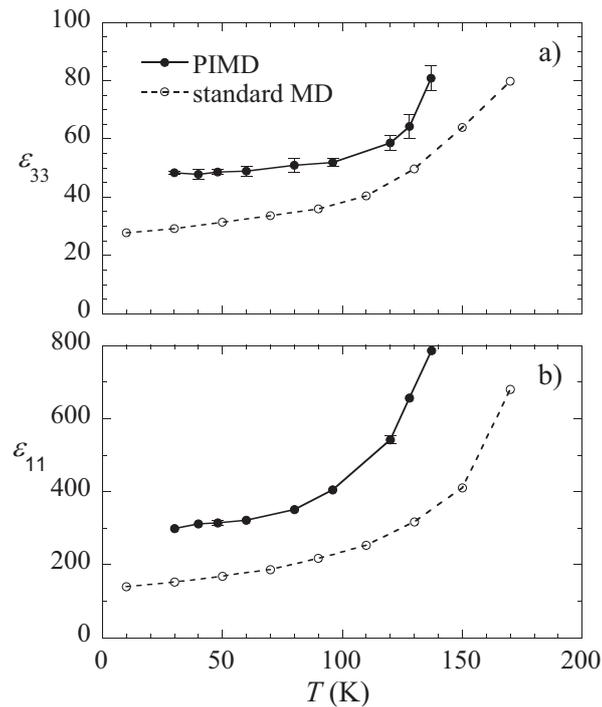
FIG. 3: Temperature evolution of the longitudinal and transverse components of the dielectric tensor, computed using either standard MD or PIMD. The electronic contribution  $\epsilon^\infty$  ( $= 5.24$  in cubic BTO<sup>13</sup>) is not included.
