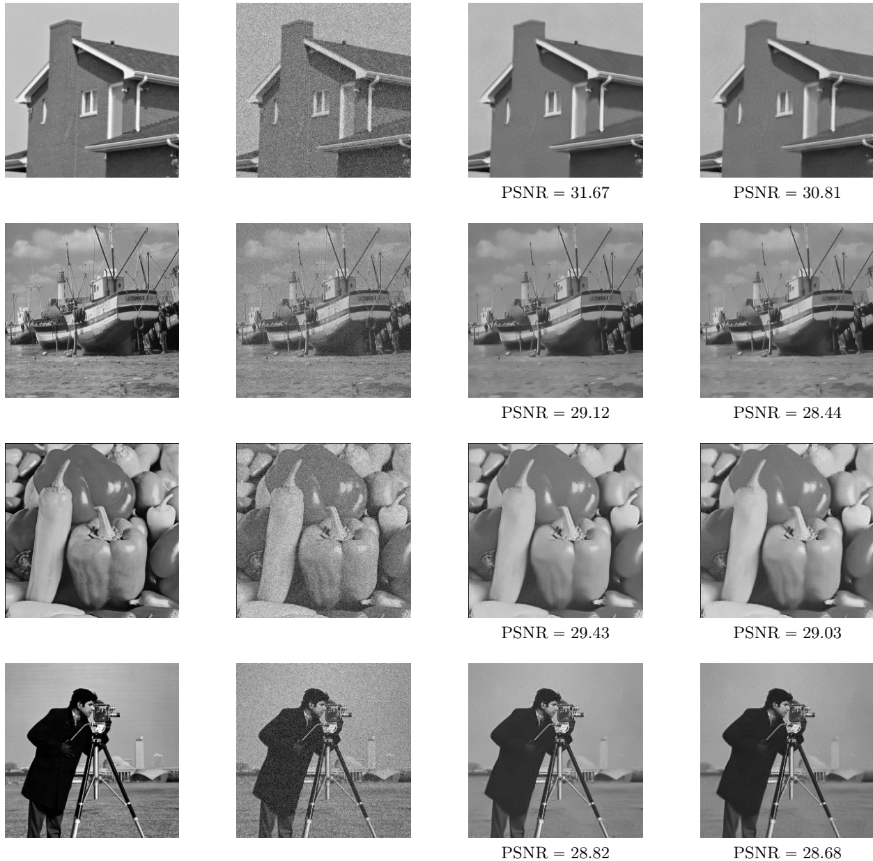
Figure 4: NL-means comparison . In this figure we compare Algorithm 2 with the traditional NL-means algorithm. Once again \omega_0 is fixed to be a 8 \times 8 square. The first column contains clean images, the second column represents the same images corrupted by a Gaussian noise with \sigma = 20 . The third column is the output of Algorithm 2 with \varepsilon fixed to 0.01 and the last column is the output of the NL-means algorithm for the optimal value of h (with regards to the PSNR). Perceptual results and PSNR are comparable, even though our algorithm yields slightly better PSNR values.
