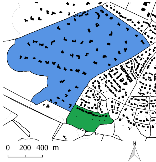
Figure 7. Example of built areas (in blue and green) with similar building density (3%) but very different spatial configuration.
