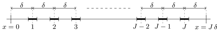
FIGURE 4. Geometry of the one-dimensional example used to study scalability of the AltMR. In this figure, \delta is the distance between the centers of the J equidistant objects that are represented by the thick segments.
