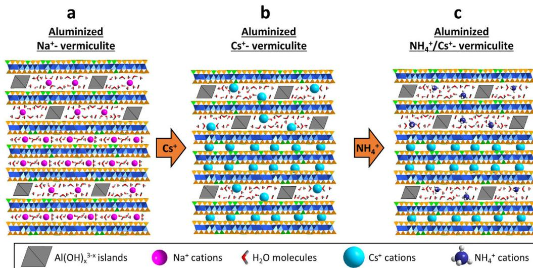
**Figure 6. The layer model for aluminized vermiculite structure and implications for Cs<sup>+</sup> mobility.**
