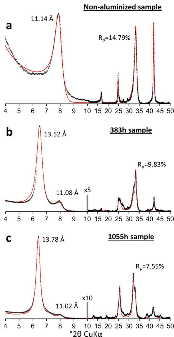
**Figure 4.** Comparison of diffraction data with the interstratified layer model of aluminized vermiculite for  $\text{Cs}^+$ -saturated specimens. The fits are performed for XRD patterns collected after  $\text{Cs}^+$  saturation of the samples shown in Fig. 2. Same notations and symbols as in Fig. 2 for original vermiculite (a) and vermiculite altered under acidic conditions for 383 h (b) and 1055 h (c).
