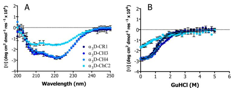
**Figure 2.** Circular dichroism spectra and chemical denaturation plots of apo  $\alpha_3$ D-CR1,  $\alpha_3$ D-CH3,  $\alpha_3$ D-CH4, and  $\alpha_3$ D-ChC2. (A) The CD spectra display two negative bands at 222 and 208 nm, demonstrating an  $\alpha$ -helical structure. (B) Guanidine hydrochloride denaturations were fit to a two-state unfolding model.
