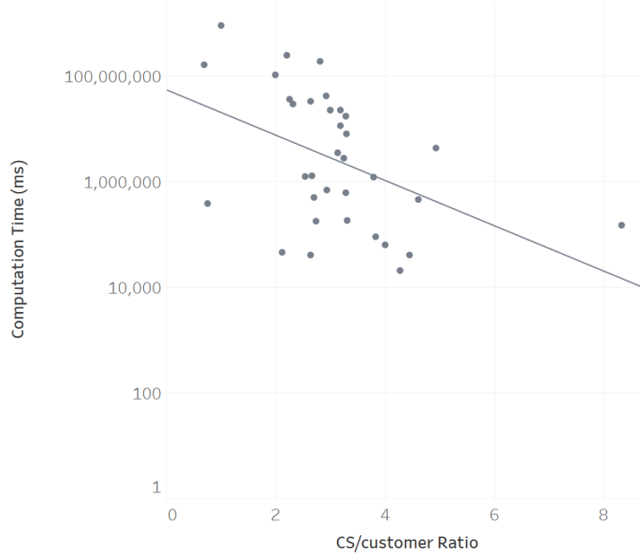
Figure 9: Computation times for instances’ PI bounds versus their ratio of CSs to customers. Note: The figure contains a point for each technician assignment, representing the sum over 50 realizations of uncertainty for each demand scenario.
