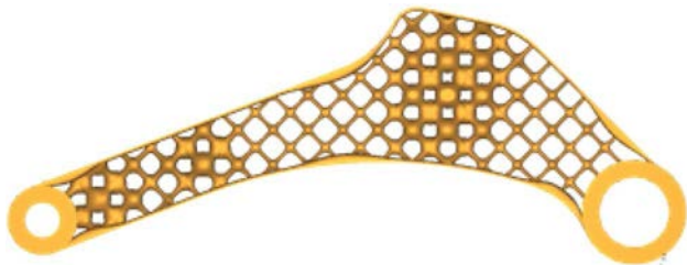
Fig. 5 Example of an optimized lattice structure using homogenized materials and preserving the topology (source Autodesk)
