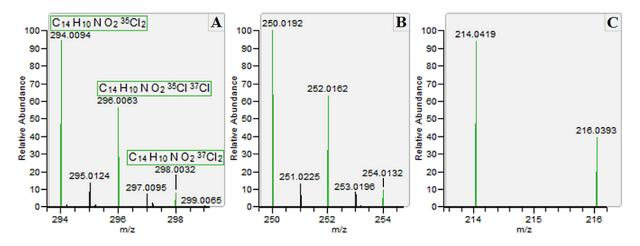
Figure 1 – High-resolution mass spectrum of DCF molecular ion at 50,000 FWHM. The green insets show the diagnostic M (m/z=294.0094) / M+2 (m/z=296.0063) / M+4 (m/z=298.0032) dichlorinated isotopic distribution (A). High-resolution mass spectrum of molecular of fragments m/z 250.0192 (B) and m/z 214.0419 (C) at 50,000 FWHM
