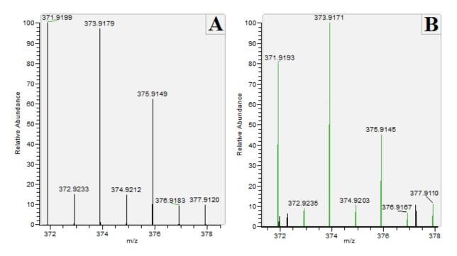
Figure 2 – Theoretical high-resolution mass spectrum of C14H10NO2BrCl2 molecular ions in negative ionization mode (A), and high-resolution mass spectrum of molecular ions of M13 at 50,000 FWHM in negative ionization mode (B)
