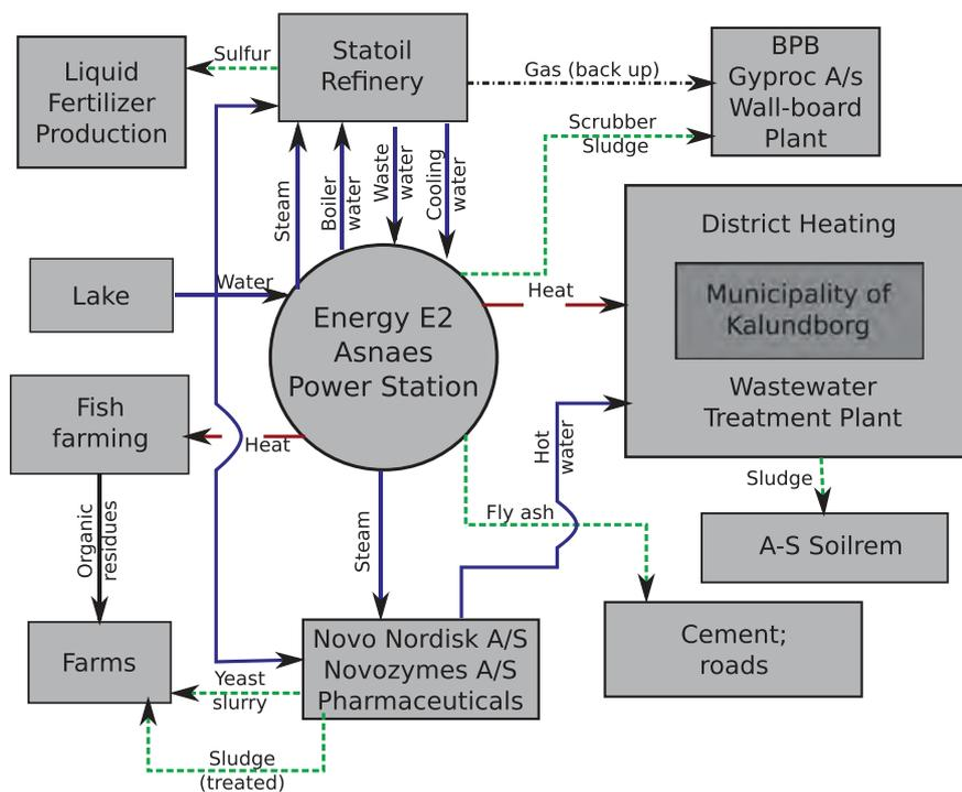
**Fig. 1.** Eco-Industrial Park in Kalundborg. Blue arrows indicate water exchanges, red arrows heat exchanges, and green arrows residue exchanges. Figure obtained from Chertow (2008). (For interpretation of the references to colour in this figure legend, the reader is referred to the web version of this article.)
