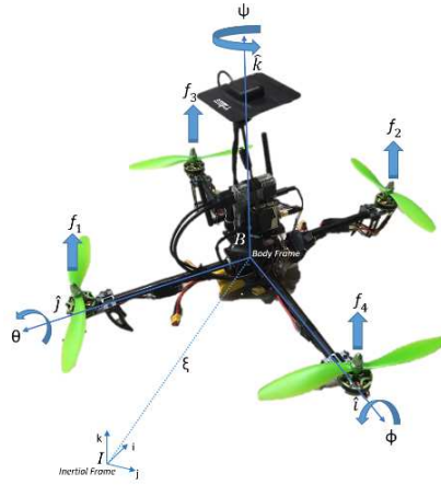
Fig. 1: Inertial and Body frame of the mini Quadrotor aircraft.
