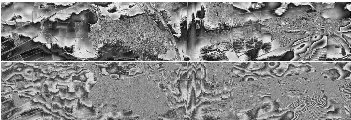
Figure 7: Interferogram from fig. 5 with phase multiplied by 5.4 (top) and 14 (bottom). The left part of the top image should look like the left part of fig. 6 while the right part of bottom image should look like the right part of fig. 6. Of course the phase detail is not exact because the baseline between take 3 and take 2 is not exactly horizontal!
