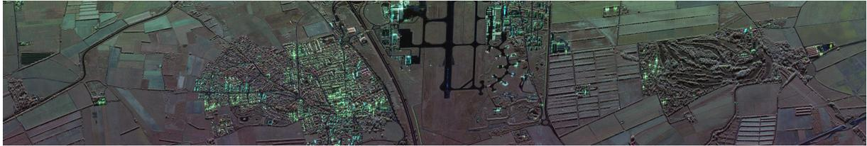
Figure 2: One of the images of the TBA dataset at X-band (flight 2, take 1) processed from raw trajectory, with Vv channel rendered as blue, Hh channel rendered as green and Hv & Vv channels rendered as red. Swath width is 1.2 km (slant), stripe length is 7.13 km. Slant range & azimuth resolutions are both 30 cm.
