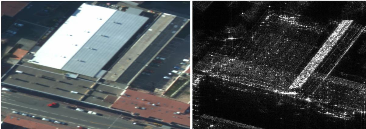
Figure 1: Example of building roof opaque in visible light (left) but transparent at X-band (right). White roofed building hosts a supermarket the aisles of which can be discerned at X-band.
