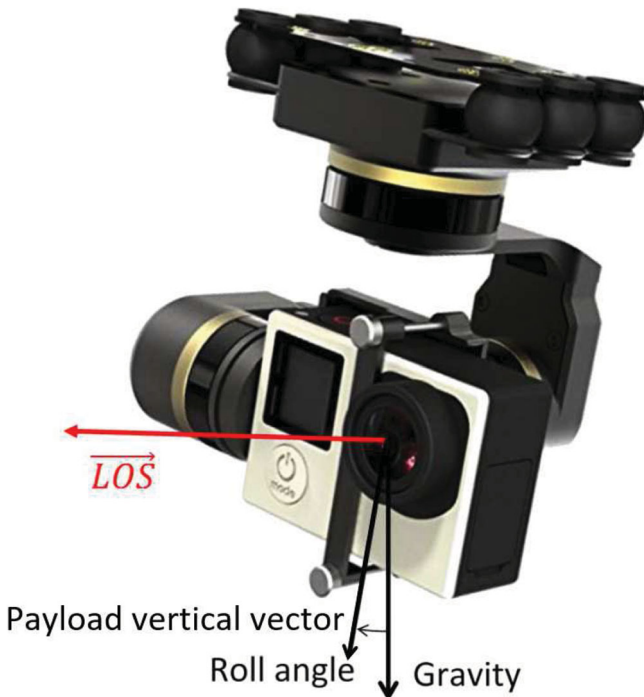
Figure 1. Gimbal attitude parameters.
