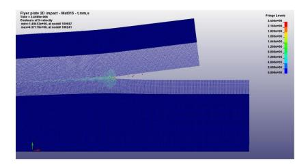
Figure 6: Velocity distribution in x direction near the collision point at 2.4989.10<sup>-6</sup> s
