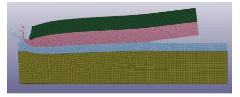
Figure 3 - LS-Dyna simulation of impact welding for a case presented in [1] at 2.4989.10<sup>-6</sup> s
