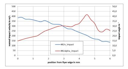
Figure 10: Evolution of the normal impact velocity (blue line) and the impact angle (red line) evaluated by the microscopic model, test #82 (from Join'EM).
