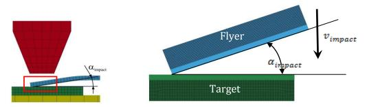
Figure 1: Geometry and initial conditions of the microscopic model
