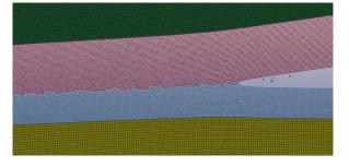
Figure 4: Wavy interface and jet at 2.4989.10<sup>-6</sup> s
