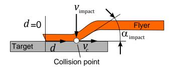
Figure 8: Definition of process parameters (from D3.1)
