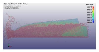
Figure 13: Performed effective plastic strain with the microscopic simulation of test #82
