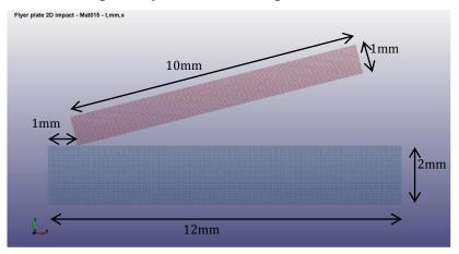
Figure 11: Geometry of the simulated case related to related to test #82
