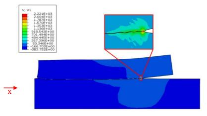
Figure 5: Velocity distribution in x-direction (from[1])
