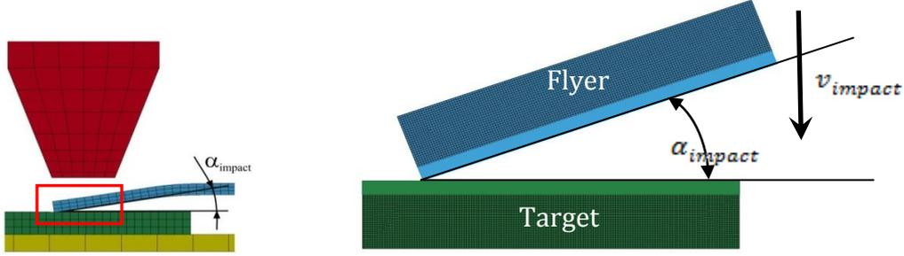
Figure 1: Geometry and initial conditions of the microscopic model
