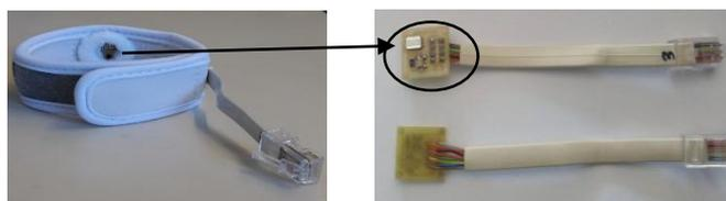
**Figure 4.** Bracelet with the three MOX sensors
