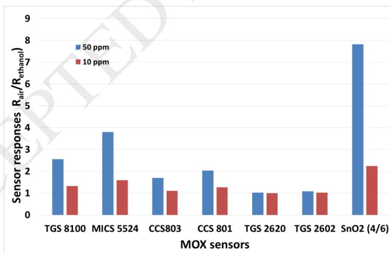
**Figure 11.** Comparison of sensors response to ethanol
