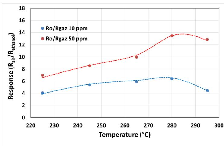
**Figure 9.** SnO<sub>2</sub> Sensor response versus temperature for ethanol concentrations with RH of 0%
