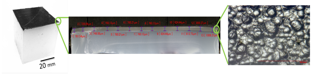
FIGURE 2 – (a) The MRE film-substrate block specimen ; (b) Microscopic topography of the MRE film-substrate block ; (c) MRE film microstructural morphology by Keyence Microscopy, 30% particle volume fraction
