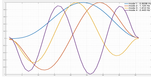
Figure 3 : First 4 mode shapes of the crest
