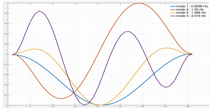
Figure 5 : First 4 mode shapes of the crest
