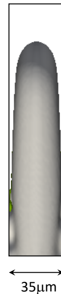
FIG. 3: Side view of the numerical domain ( 35\mu\text{m} in thickness) showing one of the two oscillating fingers intersected by the yz plane that passes through its tip. The tip radius of curvature is roughly equal to 11.5\mu\text{m} here.
