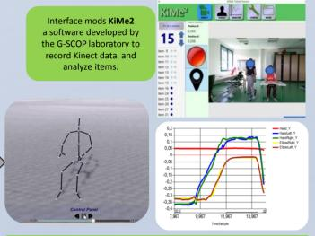
Kinect data recorded are converted into biomechanical observables on kinematic graphs and 3D reconstruction allowing the item scoring using different data (angles, distances...)
