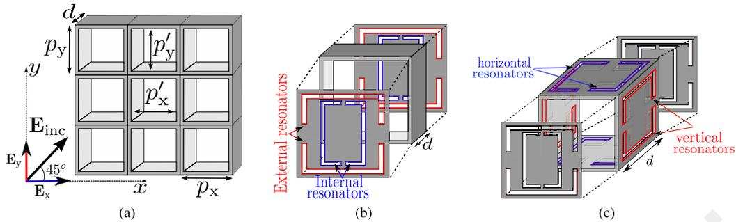
Fig. 1. Building full-metal self-supported polarizers. (a) Illumination by a  $45^\circ$ -slant plane wave of the elementary bidimensional structure. Exploded view of 3-D unit cells. (b) Simple polarizer topology. (c) Structure with enhanced performance.
