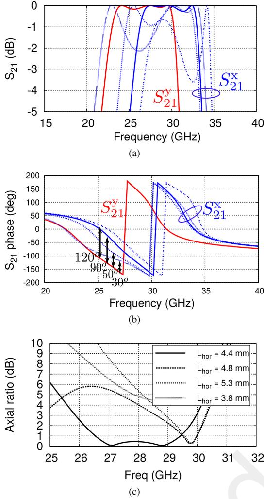
Fig. 10. Illustration of the procedure to design a polarizing 3-D unit cell using the analytical CM of Fig. 9(b). (a) and (b) Magnitude and phase of the transmission coefficient when illuminated by  $x$ - $y$ -polarized waves. (c) AR obtained when the cell is illuminated by a  $45^\circ$ -slant wave. Geometrical parameters are as follows:  $p_x = p_y = 6$  mm,  $p'_x = p'_y = 5$  mm,  $d = 1.75$  mm,  $L_{\text{ext}} = 7.5$  mm,  $L_{\text{int}} = 6.35$  mm, and  $L_{\text{ver}} = 5.5$  mm.
