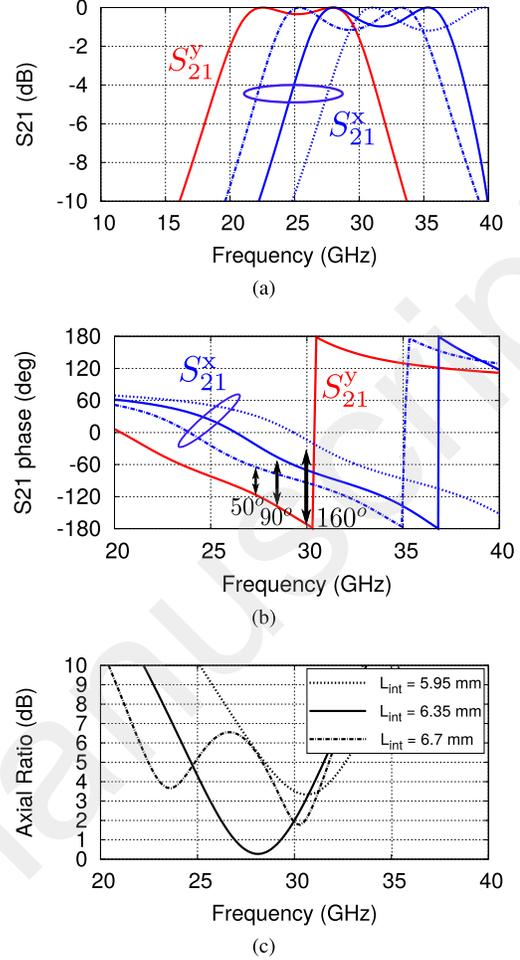
Fig. 6. Illustration of the procedure to design a polarizing 3-D unit cell using the analytical CM of Fig. 5. (a) and (b) Magnitude and phase of the transmission coefficient  $S_{21}^x$ ,  $S_{21}^y$  when illuminated by  $x$ -/ $y$ -polarized waves, respectively. (c) AR obtained when the cell is illuminated by a  $45^\circ$ -slant wave. Dimensions (in mm) are as follows:  $p_x = p_y = 6$ ,  $p'_x = p'_y = 5$ ,  $d = 1.75$ , and  $L_{\text{ext}} = 7.5$ .
