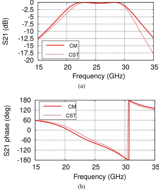
Fig. 7. Numerical comparison of the results provided by the CM and CST. Geometrical parameters are as follows:  $p_x = p_y = 6$  mm,  $p'_x = p'_y = 5$  mm,  $d = 1.75$  mm,  $L_{ext} = 7.5$  mm, and  $L_{int} = 6.35$  mm. Transmission coefficient: (a) magnitude and (b) phase.
