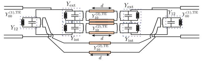
Fig. 5: Analytical CM to characterize the excitation of the 3D unit-cell in Fig. 1b considering a dual-resonance profile  $E_{\text{dual}}$  in the folded dual-slot.
