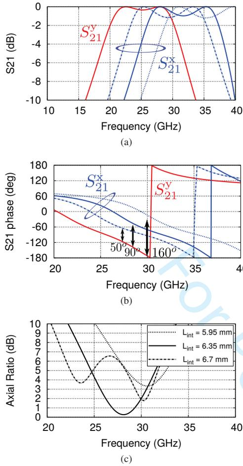
Fig. 6: Illustration of the procedure to design a polarizing 3D unit-cell using the analytical CM of Fig. 5. (a) and (b) show the magnitude and phase of the transmission coefficient  $S_{21}^x, S_{21}^y$  when illuminated by  $x/y$ -polarized waves respectively. (c) Shows the AR obtained when the cell is illuminated by a  $45^\circ$ -slant wave. Dimensions (in mm) are:  $p_x = p_y = 6$ ,  $p'_x = p'_y = 5$ ,  $d = 1.75$ ,  $L_{ext} = 7.5$ .
