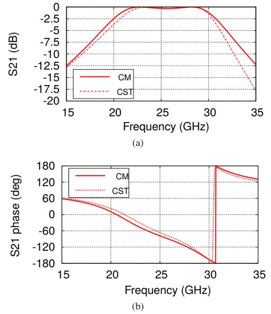
Fig. 7: Numerical comparison of the results provided by the CM and CST. Geometrical parameters:  $p_x = p_y = 6$  mm,  $p'_x = p'_y = 5$  mm,  $d = 1.75$  mm,  $L_{ext} = 7.5$  mm,  $L_{int} = 6.35$  mm.
