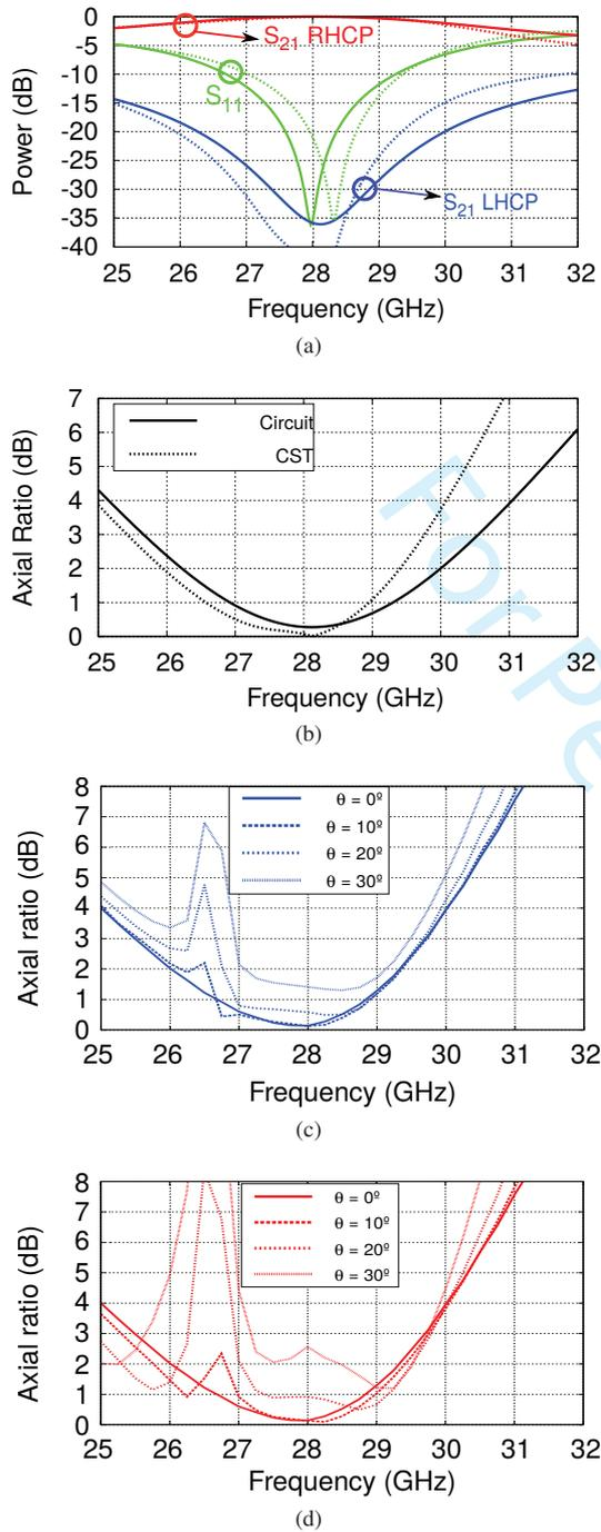
Fig. 8: Performance of polarizer designed to operate around 28 GHz. (a) Matching and transmission coefficients, comparison between CM and CST (b) Axial ratio for normal incidence, (c) Axial ratio for TE oblique incidence, (d) AR for TM oblique incidence. Geometrical parameters:  $p_x = p_y = 6$  mm,  $p'_x = p'_y = 5$  mm,  $d = 1.75$  mm,  $L_{\text{ext}} = 7.5$  mm,  $L_{\text{int}} = 6.35$  mm.
