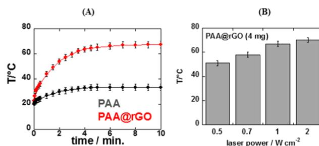
**Figure 3.** Photothermal properties of cross-linked PAA@rGO: (A) photothermal heating curves of PAA (gray) and PAA@rGO (red) nanofiber patches (4 mg) immersed in PBS (0.1 M, pH 7.4) and irradiated at 980 nm (1 W cm<sup>-2</sup>) for 10 min and (B) temperature profile of PAA@rGO nanofiber mats upon 10 min irradiation at varying power densities.
