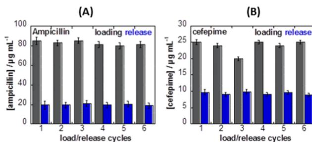
**Figure 7.** (A) Loading of ampicillin ( $85 \mu\text{g mL}^{-1}$ ) and the amount of photothermally released ampicillin after 10 min laser irradiation ( $1 \text{ W cm}^{-1}$ ). (B) Loading of cefepime ( $25 \mu\text{g mL}^{-1}$ ) and release of cefepime when activated at  $980 \text{ nm}$  at  $2 \text{ W cm}^{-2}$ .
