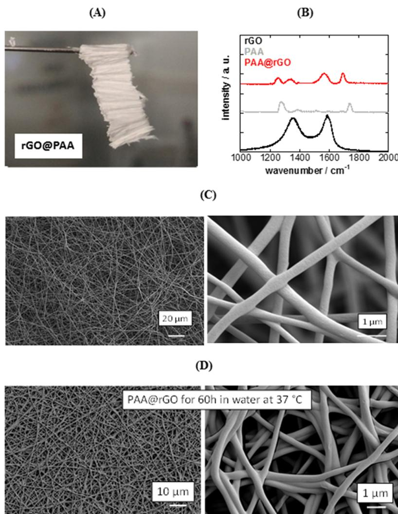
**Figure 2.** Characterization rGO-loaded PAA nanofiber mats formed by electrospinning: (A) photograph of electrospun PAA@rGO; (B) Raman spectra of rGO (black), PAA (gray), and PAA@rGO (red); (C) scanning electron microscopy (SEM) images of fabricated PAA@rGO nanofiber mats at different scales; and (D) stability of  $\beta$ -cyclodextrin cross-linked PAA@rGO nanofibers in water at 37 °C for 60 h.
