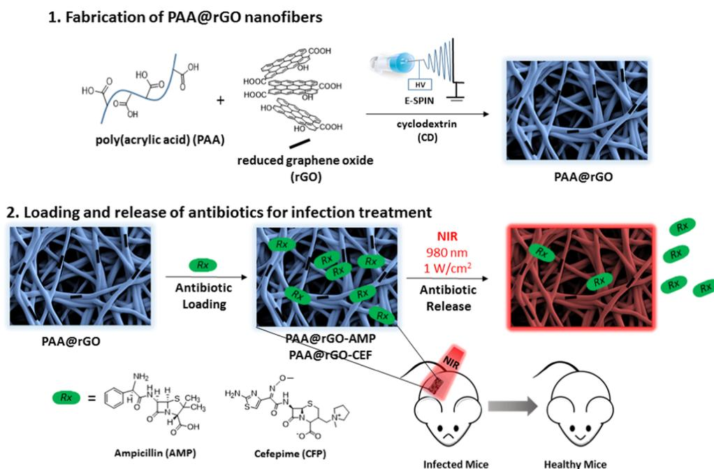
**Figure 1.** Illustration of the fabrication of antibiotic-loaded PAA@rGO nanofibers: (1) electrospinning of rGO-loaded PAA nanofiber mats followed by (2) loading with different antibiotics and photothermal-triggered antibiotic release.
