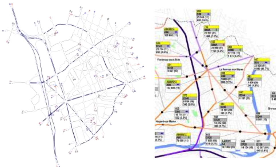
Figure 1: Network of the traffic microsimulation (left) ; traffic experimental data (right) - Trafipollu project
