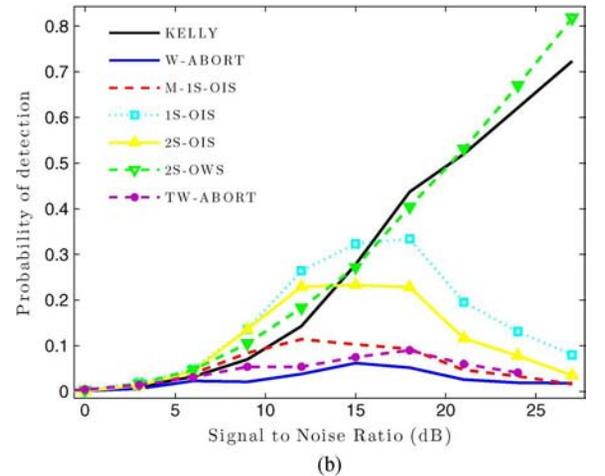
Fig. 3. Probability of detection under mismatched conditions for  $T = 2M$  ( $\delta f_\nu = 0.5/M$ ). (a)  $p = 0.1$ ; (b)  $p = 0.9$ .
