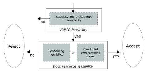
Figure 2: Logical flow-chart of feasibility tests for the VRPCD-RC
