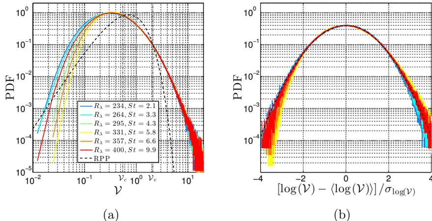
Figure 3: (a) Probability distribution of normalized Voronoï area  $\mathcal{V}$  for experiments at different Reynolds number and Stokes number. The red dashed line represents a random Poisson process (RPP) distribution. (b) Probability distribution function, centered and reduced, of  $\log(\mathcal{V})$  for the same experiments as in figure (a). The black dashed line represents a Gaussian distribution.
