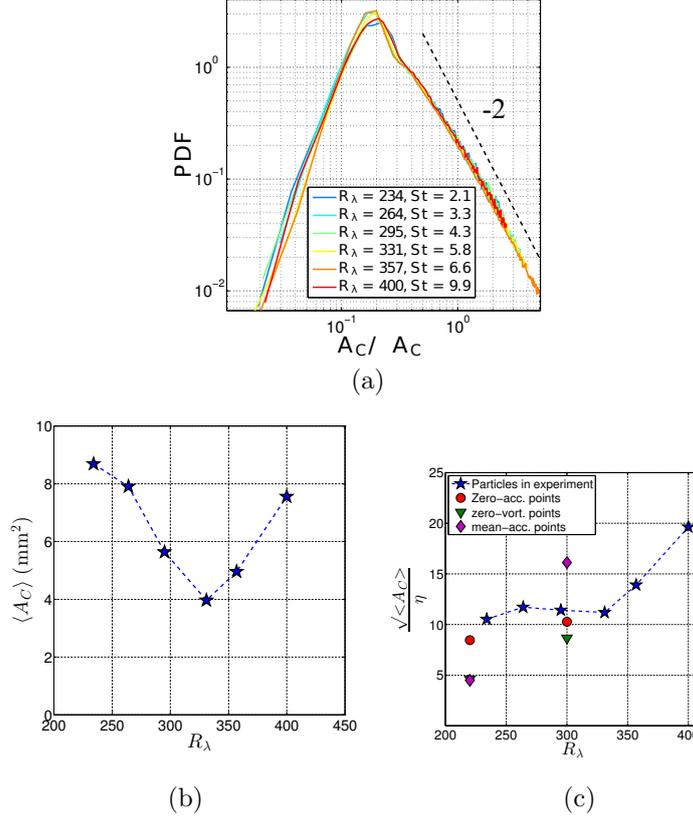
Figure 5: (a) PDFs of clusters area normalized by the mean. (b) Mean value of clusters area as a function of  $Re_\lambda$ . (c) Linear dimension of clusters normalized by the dissipation scale of the flow. Red circles represent the value obtained numerically in section 3 for clusters of *zero-acceleration points*, the green square is for clusters of *zero-vorticity points* and the magenta diamond for clusters of *mean-acceleration points*.
