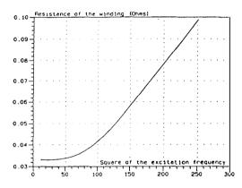
Fig. 2. The ac resistance of the studied winding in function of the square of the excitation frequency.
