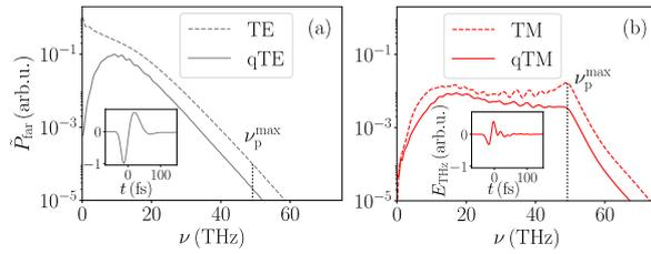
**Fig. 2.** Experimental THz spectra for qTE (a) and qTM (b) polarization (see text for details). Corresponding on-axis THz waveforms are shown as insets. The dashed lines specify the estimated maximum plasma frequency.
