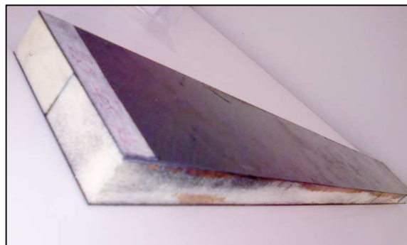
Figure 8: Fully coupled sandwich beam ready to be tested
