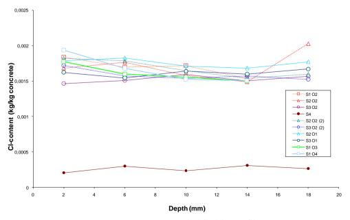
Figure 1. Total chloride profiles
