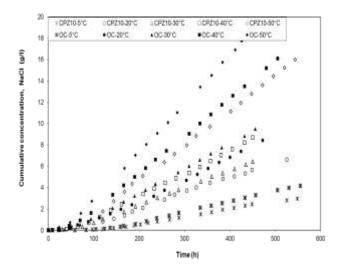
2 Fig. 3–Evolution cumulative increase of chloride concentration in downstream cell
