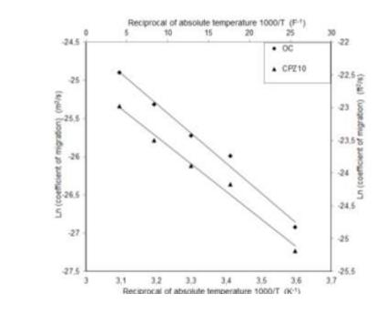
Fig. 7–Arrhenius plots of the diffusivity in concrete mixtures.
