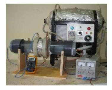
Fig. 2–Migration cell with hot and cold device.
