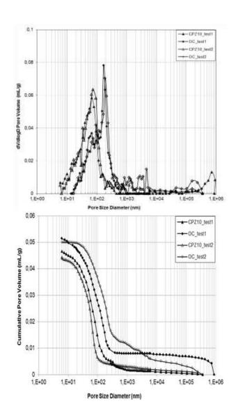
Fig. 4–Measured porosity in OC and CPZ10 specimens using MIP test (Note : 1 nm =
