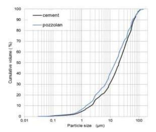
Fig. 1– Laser granulometry of Cement and Natural pozzolan (Note :  $1 \mu m = 3.937 \ 10^{-5}$
