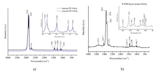
Fig. 3. Raman spectra of non-sterilized films of internal and external PE bag layer (a); EVOH layer and additives (b). The stars stand for the fingerprints of the additives.
