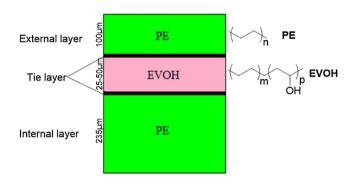
**Fig. 1.** Molecular structure of PE-film. The internal layer is the side of the film in contact with the solution when the bag is filled. The external layer is the side of the film in contact with air. The tie layer is used to glue PE and EVOH layers together.
