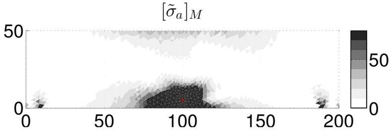
**Figure 6:** Contour plot of the asymptotic approximation in terms of equivalent (Mises) stress perturbation  $[\tilde{\sigma}_a]_M$  with the varying flaw  $\mathbf{z}$ , and fixed evaluation point  $\mathbf{x} = (100, 5)$  denoted with  $+$ . The flaw is taken as elliptic hole with the semi-axes ratio  $a_1/a_2 = 8$ , and principal axes rotated with respect to global coordinate system for  $\theta = 45^\circ$ . The stress perturbation is given in MPa.
