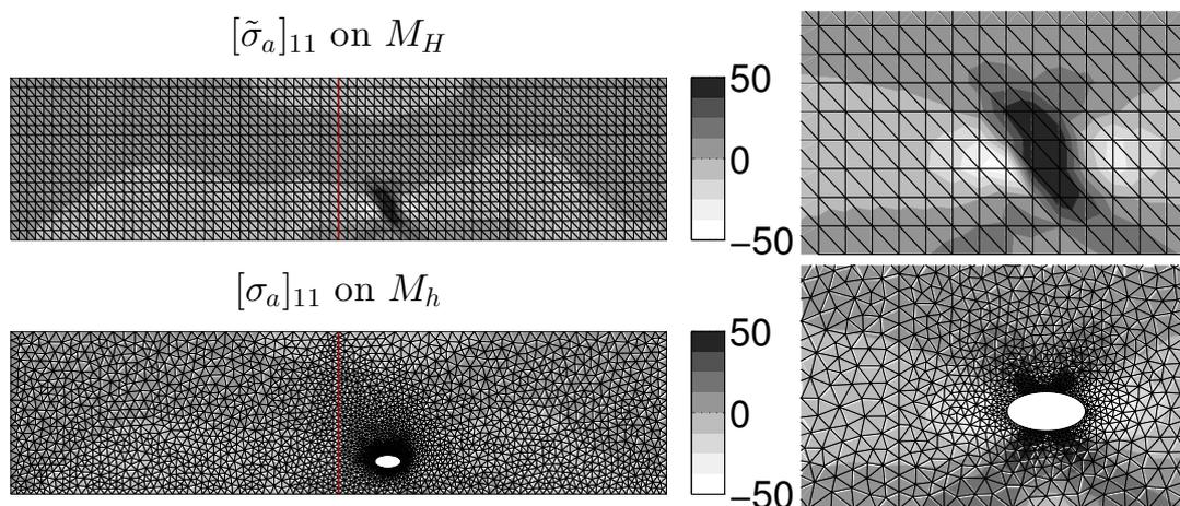
**Figure 4:** Contour plots of the asymptotic approximation  $\tilde{\sigma}_a^H$  of the stress perturbation (upper plots) and the reference perturbation  $\sigma_a^h$  (lower plots). The plots on the right are zooms showing both fields in the vicinity of  $\mathbf{z}$ . The elliptic hole is located at  $\mathbf{z} = (115, 10)$ , and its inclination is  $\theta = 0$ .
