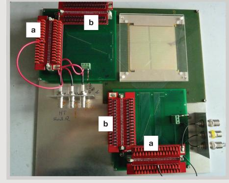
Fig. 7. Electronic card built in order to test the leakage current of the DSSD. The top card on the left is used to measure the n-side and the bottom card on the right is used to measure the p-side. The (a) pins are used to input the high voltage and the (b) pins are used to extract the signal.
