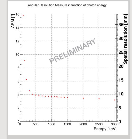
Fig. 6. Variation of the Compton camera's ARM versus the different monoenergetic photon energies. The fit of the ARM distribution is calculated by the Voigt function. The right scale is an estimation of the spatial resolution. In order to estimate this resolution, it uses a point of interaction in the scatterer located in the middle of the stack (135 mm from the source).
