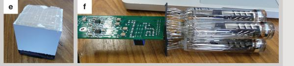
Fig. 5. a. The hodoscope **b.** 2 PMs Hamamatsu H8500 connected via optic fibers (on each side) c. DSSD mounted on an electronic card **d.** First prototype of an ASIC of the DSSD's front end e. Block BGO (100 blocks compose the absorber) **f.** Each block is connected to 4 PMs
