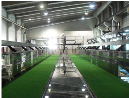
Fig. 1. Compound open-channel flume (18m × 3m), Irstea Lyon-Villeurbanne, France.
