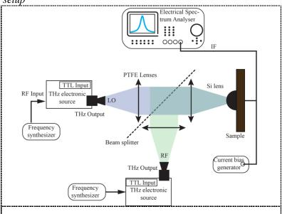
**Figure 1.** Heterodyne detection set-up using two electronic sources.
