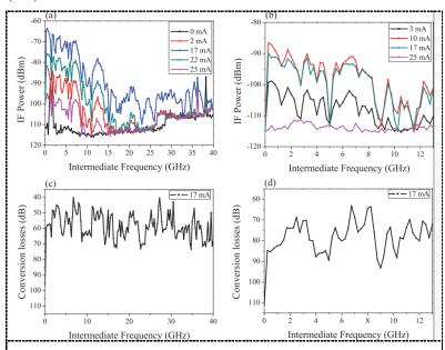
**Figure 2.** Experimental IF power measured for different bias current, with RF and LO belonging to the frequency ranges (a) 0.300 THz and (b) 0.650 THz. (c) and (d) show the corresponding conversion losses for I = 17 mA.
