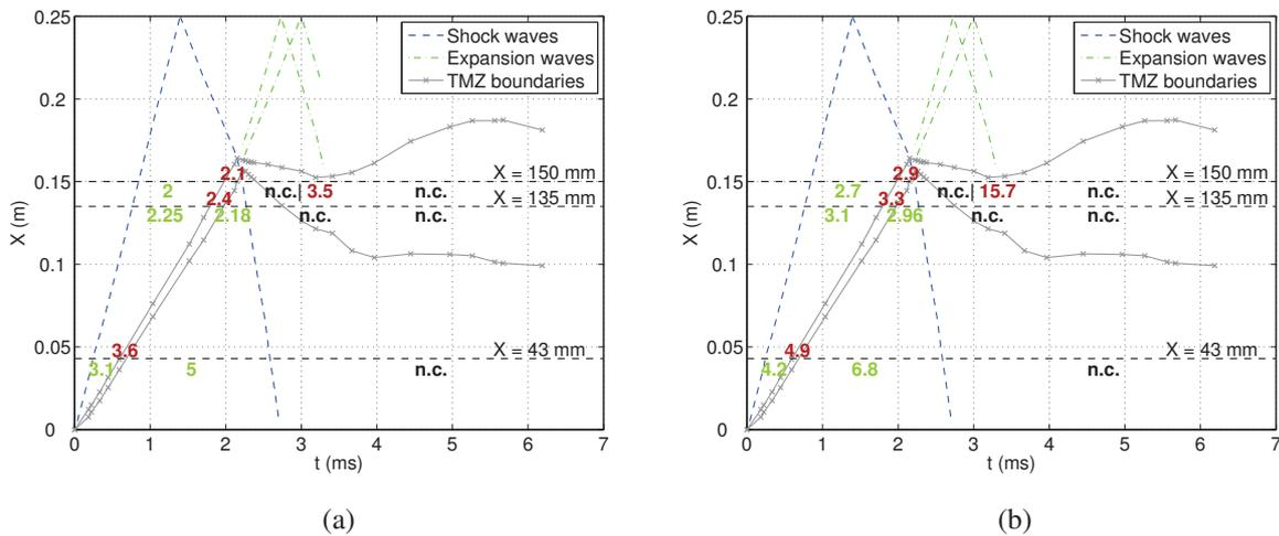
Fig. 14. Experimental ( $X - t$ ) diagram of an Air/SF<sub>6</sub> mixing configuration (Conf4) and associated measured (a) fluctuations (m/s), (b) turbulence intensity (%). Green and purple numbers correspond to statistically converged or indicative values of the turbulence levels respectively. ‘n.c.’ refers to non-converged values.
