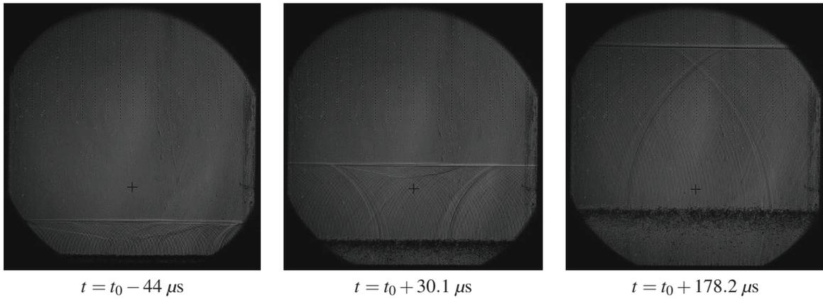
Fig. 9. Schlieren images of the perturbations generated by the shock wave in pure air configuration (Conf3). The black cross on the images indicates the location of the LDV probe volume at  $X = 43$  mm. The origin of time on the figure corresponds to the instant of passage  $t_0$  of the incident shock wave on the LDV probe volume. Here the dark zone corresponds to membrane fragments.
