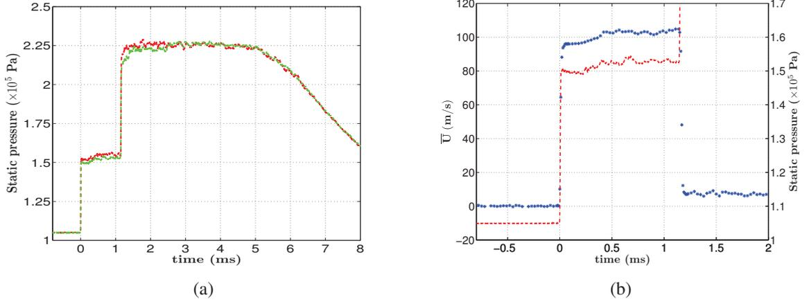
Fig. 6. (a) PPT3 static pressure signals ( $X=43$  mm above the interface) for Conf1 (green) and Conf2 (red) over the whole phenomenon history ; (b) Concurrent evolutions of the mean  $X$ -velocity (blue symbols) and PPT3 static pressure (red dashed line), zoomed around the velocity plateau between the incident and reflected shock waves for Conf2. The origin of time on the figure corresponds to the instant of passage  $t_0$  of the incident shock wave on the LDV probe volume at  $X = 43$  mm.
