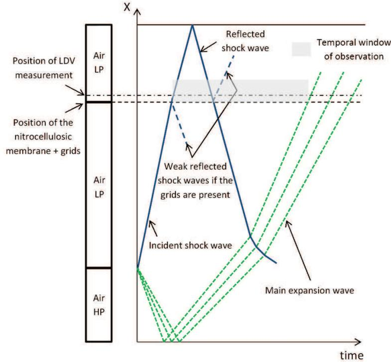
Fig. 3. Schematic ( $X-t$ ) diagram representative of an homogeneous experiment
