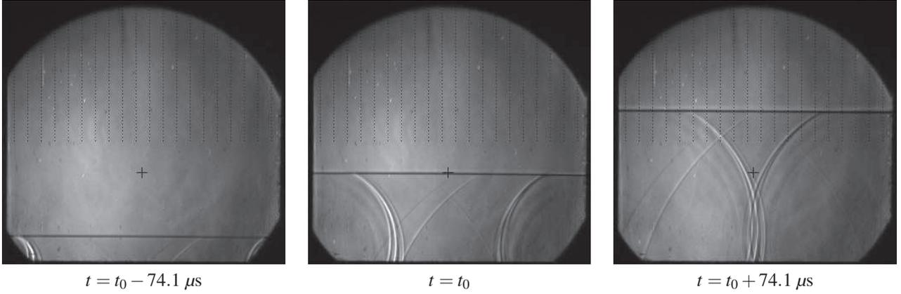
Fig. 7. Schlieren images of the perturbations generated by the shock wave in pure air (Conf1). The black cross on the images indicates the location of the LDV probe volume at  $X = 43$  mm. The origin of time on the figure corresponds to the instant of passage  $t_0$  of the incident shock wave on the LDV probe volume.
