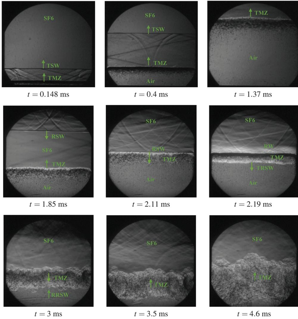
Fig. 11. Illustration of the TMZ evolution (Conf4). The reader can refer to Fig. 10 for the definition of acronyms.
