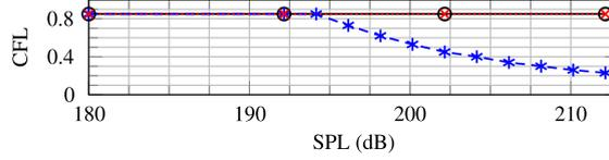
**Fig. 5.** Maximum CFL number against SPL for the impedance tube of Fig. 4. (—○—) Hard wall  $\mathcal{B}$ -flux and DG4-RKF84- $\mathcal{B}$ -flux. (- \* -) Nonlinear model (23) with  $(a_0, C_{nl}) = (0, 1)$  and DG4-RKF84- $\mathcal{Z}$ -flux. (···×···) Same nonlinear model with DG4-RKF84- $\mathcal{B}$ -flux.
