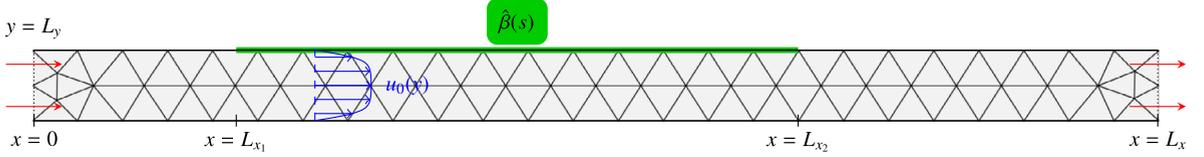
**Fig. 6.** Flow duct considered in Sec. 6 (aspect ratio of the GIT). Mesh of 106 triangles used in Fig. 14. Pressure measurements are taken on the lower wall  $y = 0$ . See Table 1 for geometrical dimensions corresponding to the GIT and GFIT.
