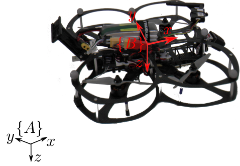
Fig. 1. Quadrotor platform: The platform used for the indoor experiments showing the body-fixed \{B\} and inertial \{A\} frames.
