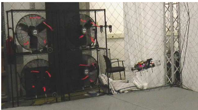
Fig. 10. Quadrotor flying in synthetic wind field for wind velocity estimation. The red streamers show the direction and strength of the airflow.
