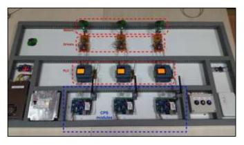
Fig. 6-The CPS prototype: three brushed motors are controlled by the PLCs; each PLC is connected with the proposed hardware to make them communicate; details in (Dassisti et al., 2017).
